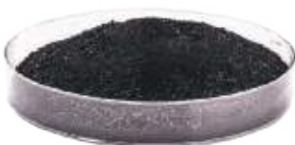
Granular activated carbon from olive pomace
